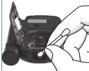
Carefully dab the measuring optics and the front opening of the meter with a slightly dampened cotton swab.
