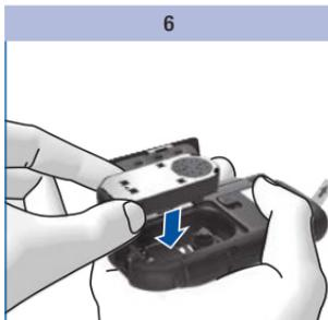
Insert the test cassette in the meter with the silver side facing upwards.
