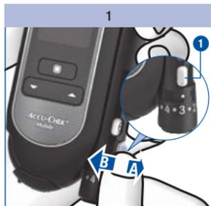
Push the lever 1 in direction A and then back again in direction B.
