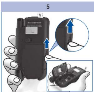
Push the slide button for the cassette compartment cover upwards in the direction of the arrow.
