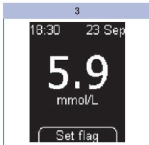
Testing is complete after approx. 5 seconds, depending on the blood glucose concentration. The test result appears on the screen and the beep tone sounds. The meter saves the test result at the same time. The used test area is transported away from the tip of the cassette.
