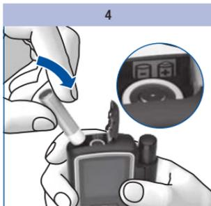
Insert two new batteries in the battery compartment. Ensure that the polarity (+ and -) of the batteries is correct.
