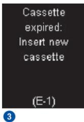
If the test cassette in the meter is empty **1** or defective **2** or has expired **3**, the appropriate message appears after the display check and the number of available tests (see also page 120). Shortly after this, the meter turns off automatically.
