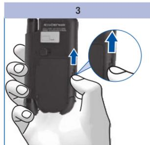
Push the slide button for the cassette compartment cover upwards.
