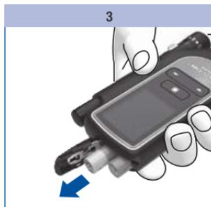
Turn the meter so that the batteries fall downwards out of the battery compartment.
