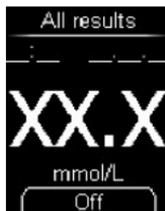
If the last (most recent) result in the memory is displayed as *XX.X mmol/L* with dashes instead of the time and date, the last test did not deliver a result. This means that during the last test either an error message was displayed or you did not apply blood (or control solution) after the prompt *Apply drop* was displayed. After the next test that delivers a result, the result displayed with X is deleted from the memory.
