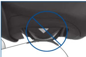
Do **not** press the test area and the finger together. Avoid trembling or shaky movements.
