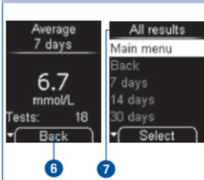
*Back* **6** (press and release the button) opens the higher-level menu **7** of the currently displayed menu.
