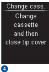
If you have prepared for the test cassette replacement via *Change cass.* the meter prompts you to replace the test cassette **4**. Shortly after this, the meter turns itself off automatically.
