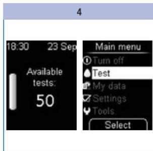
The meter displays the number of tests in the test cassette that are still available.
