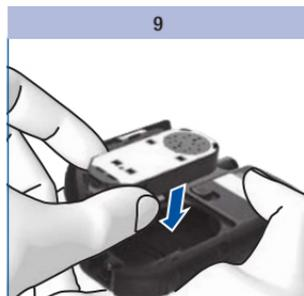
Re-insert the test cassette in the meter.
