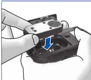
Insert the new test cassette in the meter with the silver side facing upwards.
