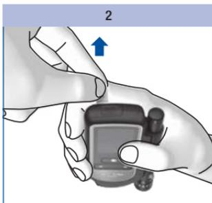
Pull the protective strip of the batteries backwards out of the meter.
