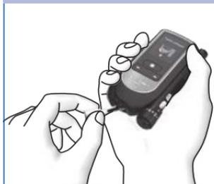
Apply the control solution to the centre of the test area at the tip of the cassette using the tip of the brush.
