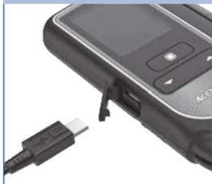
Plug the Micro B connector of the USB cable into the USB port on your meter.
