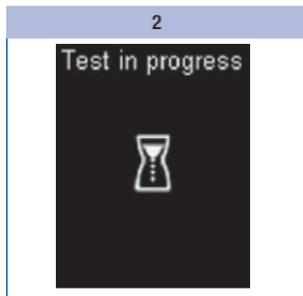
Remove your finger from the test area when the beep tone sounds and *Test in progress* is displayed.
