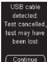
If you connect the meter to a PC while a test is in progress, the test is cancelled and a message appears on the screen.
