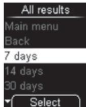
Use ▼▲ to select the time period in which the test results were obtained: *7*, *14*, *30* or *90 days*.
