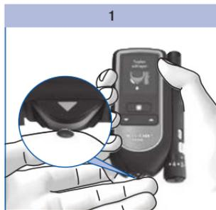
Apply the blood drop to the centre of the test area.
