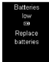
This message appears when the batteries are almost empty. It appears every time you turn the meter off if you have not yet changed the batteries. After the message appears for the first time, you can still perform about 50 tests.
