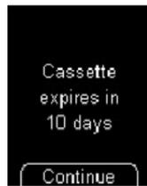
This message appears at the start of a test if the test cassette is only valid for 10 more days. The message is repeated when the test cassette is only valid for 5, 2 and 1 more day(s).
