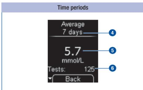
You can choose which test results are used for calculating the averages:
